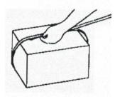
Place the strap around the material with the end of the strap at the bottom as in the picture. The part that goes around the material should be on top.
